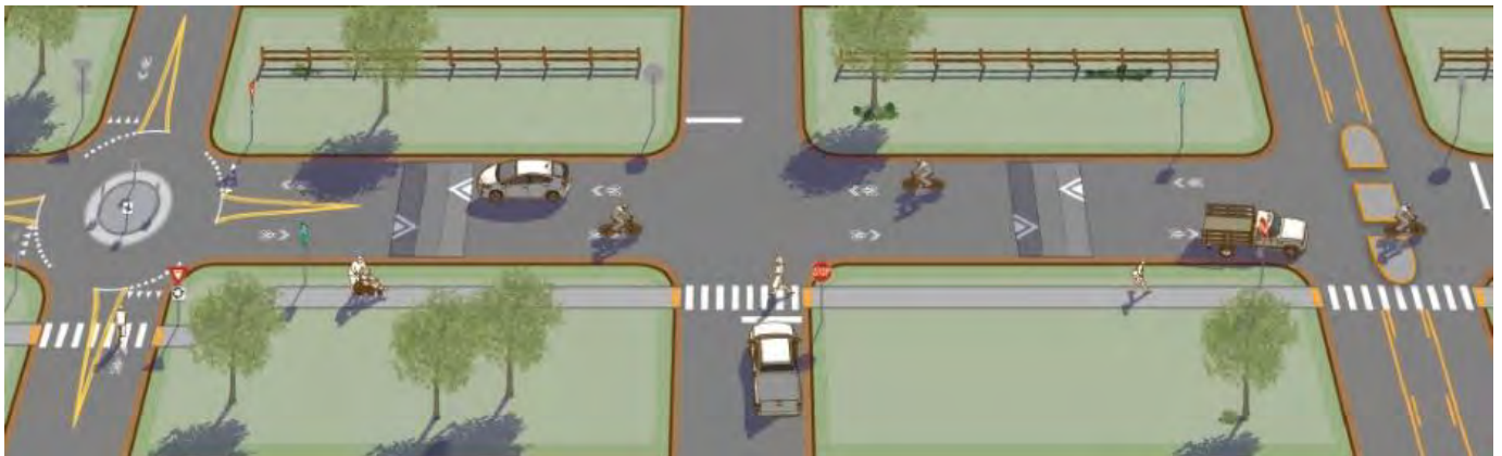
Example layout of a bicycle boulevard that shows a refuge island, speed humps, and a roundabout (Source: FHWA, Small Town and Rural Multimodal Networks )
