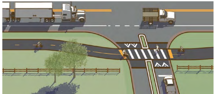
Example layout of a sidepath adjacent to a busy roadway as it crosses a perpendicular street. (Source: FHWA, Small Town and Rural Multimodal Networks )
